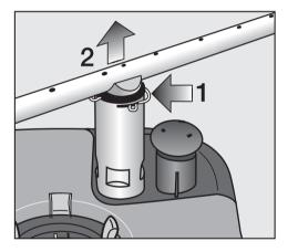
■ Loosen the securing clip on the spray arm connection and then pull the spray arm upwards or downwards.
